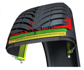
The multi-radius cavity with a small shoulder radius ensures a long, wide footprint that delivers more even pressure distribution between the tire and the road surface. This ensures that the UltraGrip Ice+ provides improved road contact, displays more even tread wear and delivers improved mileage levels.
